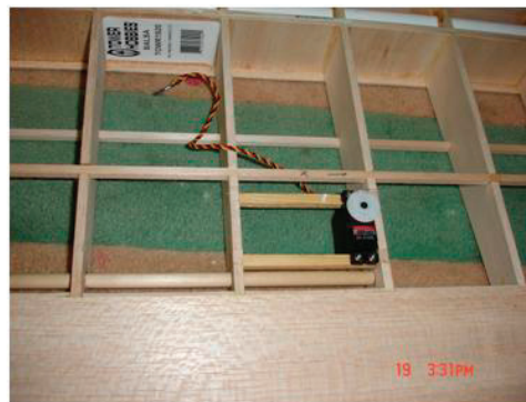
Fig. 4. Servo motor mounted to the wing.
