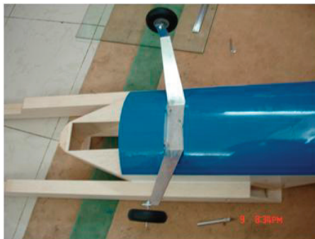
Fig. 9. Landing gear mounted on the fuselage.
