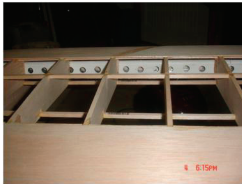
Fig. 3. Aluminum spar in the wing.
