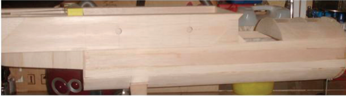
Fig. 7. Fuselage and the tail boom mounted .
